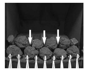
e) Select five of the large coals and arrange along the rear of the fuelbed, using the ribs in the rear of the fuelbed as a guide for placement. (See fig. 7 below)
